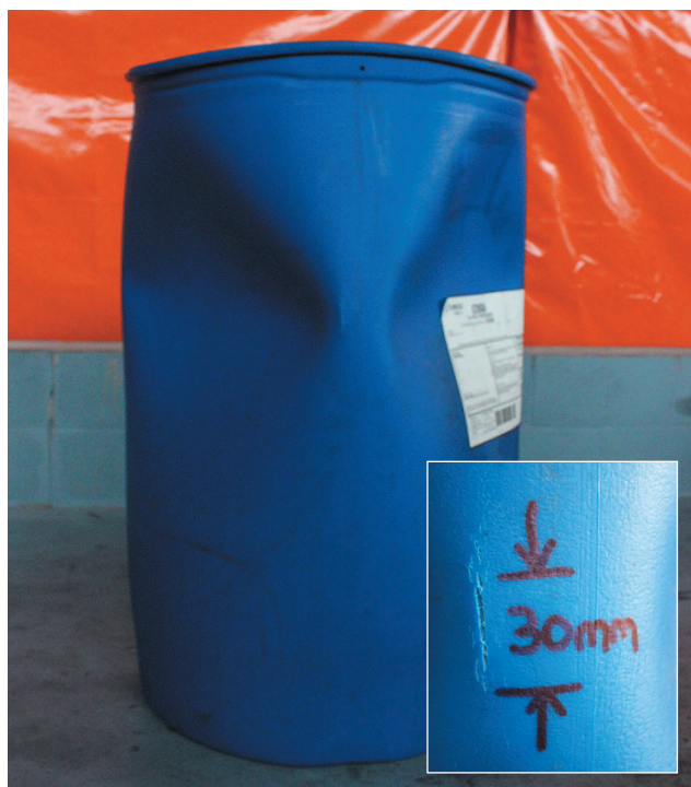
An 18-year-old plastic drum with deformation presumed to be through loss of solvent. Inset shows a resulting crack, which ultimately led to a leak in the drum.
