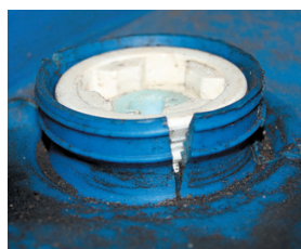
Splitting necks were observed on 25% of this stockpile of plastic drums after 10–20 years in storage. The specific cause was not known, but such damage could have an adverse impact on the product as it is likely to become exposed to the air.
