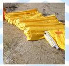
Caution The attachment points for anchor lines are at the waterline on the boom connectors. Do not attach anchor lines to the handholds or ballast chain.
