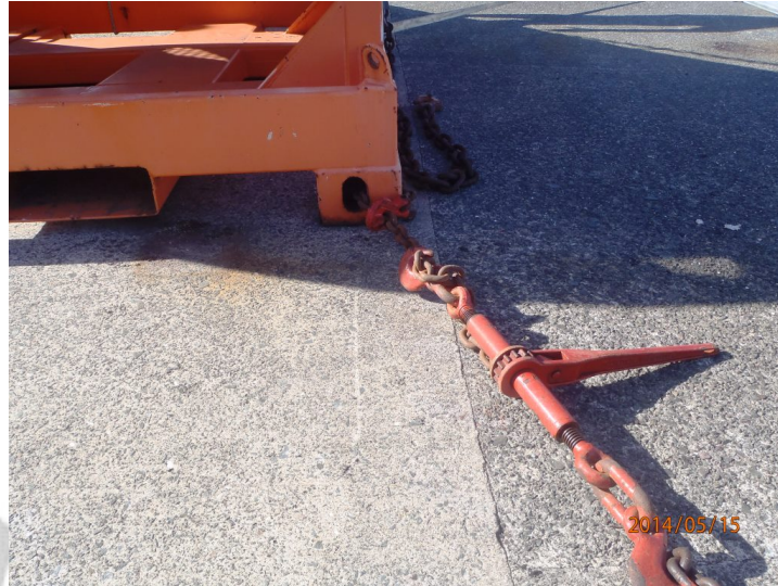
Chain and ratchet technique to secure reel to deck
