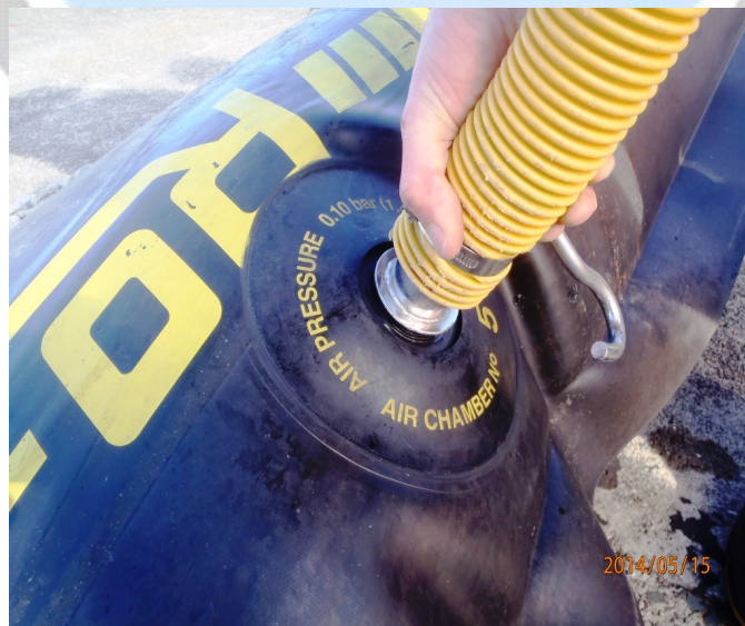
Inflation hose in place
