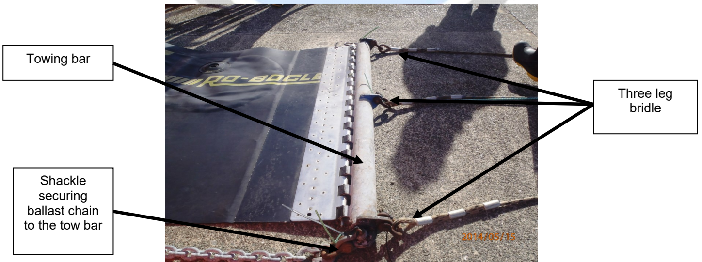
Towing bridle configuration
