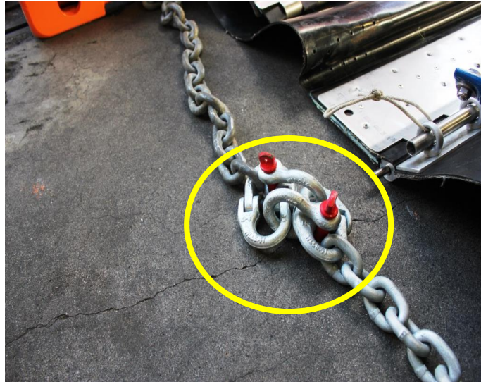
Example of correct technique to connect two ballast chains
