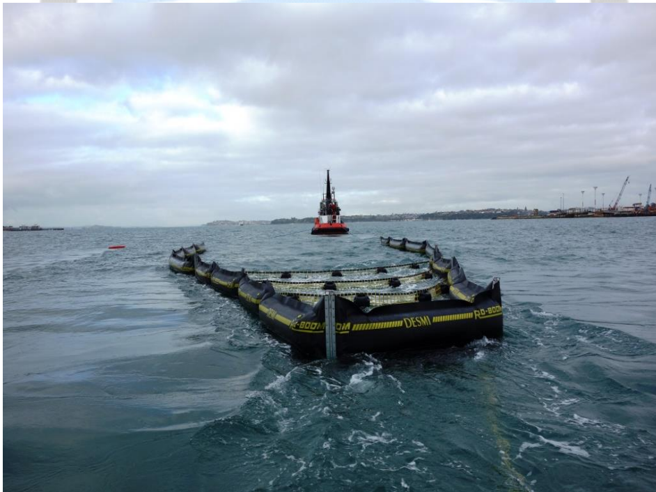
Speed Sweep deployed and in tow (vessel and boom vane)
