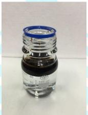
Measure 20ml of oil and apply with syringe to surface of water. Apply dispersant by evenly dripping over the surface of the oil.
