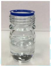
**B.**Fill test jar with 80ml of fresh seawater.
